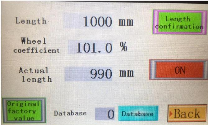
Length: input how long you want to cut the cable and press “length confirmation”
