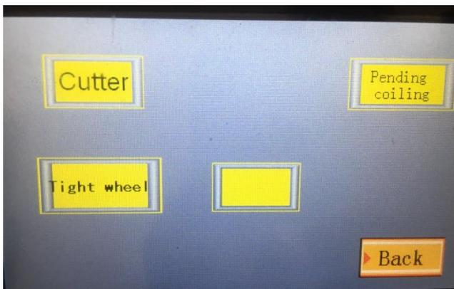
Cutter: cut the cable manual
