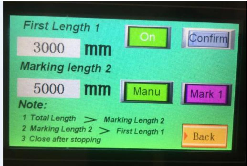
First length 1: the length is first length that cable output
