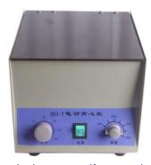
This electric laboratory centrifuge is a desktop centrifuge and widely applied in biological, chemical, pharmaceutical and other research and production departments of education, its maximum speed could reach 4000 rpm/min for the separation and identification and radioimmunoassay cells and large particles and so on.
