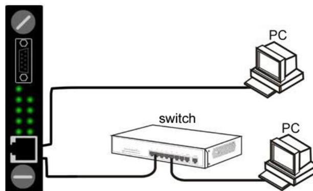
Figure 1-1 Cable Connection between PC and Management Card
