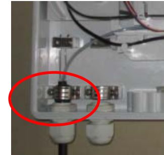
Step 1: Insert small diameter cable and fix it.
